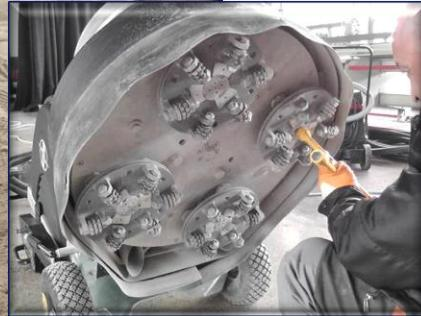
Concrete roughening is used to remove the smaller irregularities of surfaces. This technology is most commonly used for removing the residual adhesive layer after the demolition of a floor cover. The same technology can be used for leveling "protruding" gravels with concrete surfaces, eliminating one of the most common defects of old concrete surfaces.
